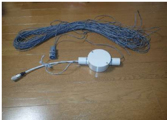
Fig. 2: An example of EFHWs antenna ( f_0=3.5\text{MHz} )
