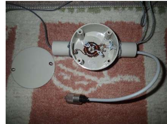
Fig. 3: Close-up of feeding point and broadband transformer.
