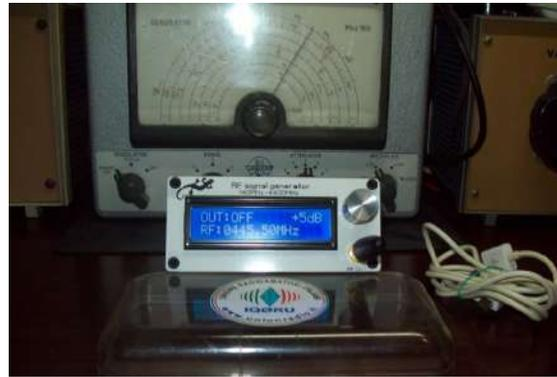
140MHZ-4400MHZ RF signal generator, signal source
